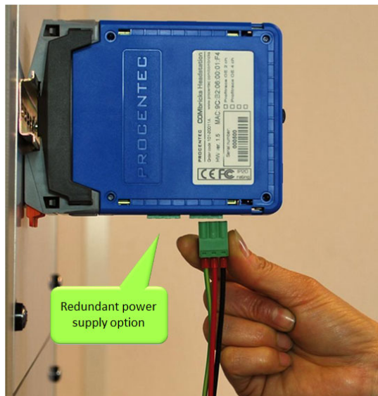
Powering the Head Station
