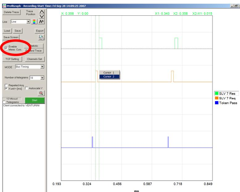
Select **Enable Meas. Curs.** Inside the graphic area, press the **right button** of the mouse and place the first and the second cursor.
